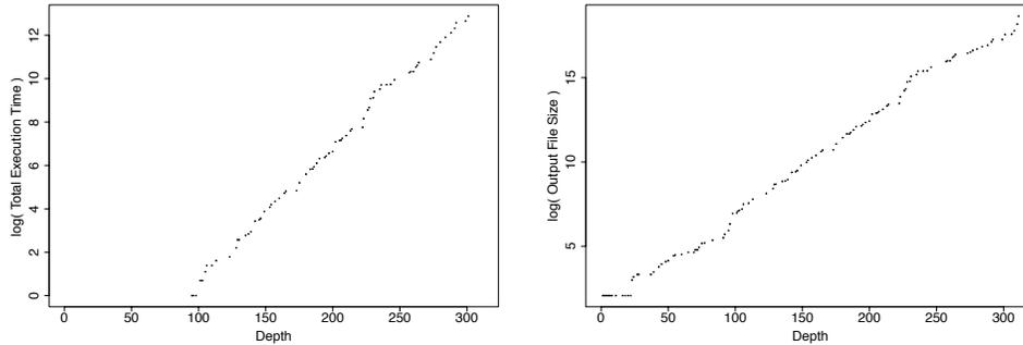
Figure 3: Log-linear plot of cumulative execution time in seconds (left) and output file size in kilobytes (right) against tree depth.
