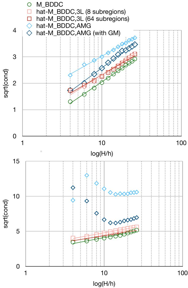
FIG. 7.1. Homogeneous linear elastic cube decomposed into 512 subdomains with  $H/h = 4, 6, \dots, 26$ . Top:  $E = 210.0$  and  $\nu = 0.3$ ; Bottom:  $E = 210.0$  and  $\nu = 0.49$ . We vary the number of subdomains per subregion in  $\hat{M}_{\text{BDDC},3L}^{-1}$ , and we compare nodal AMG and AMG-GM in  $\hat{M}_{\text{BDDC},\text{AMG}}^{-1}$ . Computed on the magnitUDE supercomputer.
