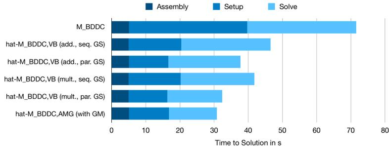
FIG. 7.5. Comparison of BDDC setup and solve times of  $M_{\text{BDDC}}^{-1}$ ,  $\widehat{M}_{\text{BDDC,VB}}^{-1}$  with different Gauß-Seidel setups and  $\widehat{M}_{\text{BDDC,AMG}}^{-1}$  with GM. Using edge translations as constraints. Homogeneous linear elastic cube decomposed into 5832 subdomains with  $H/h = 22$ . Corresponding weak scaling experiments can be found in Figure 7.4. Computed on magnitUDE supercomputer.
