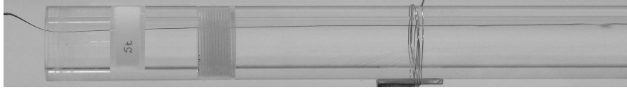
FIG. 2.3. No vena contracta at a sharp edged entrance in our color band experiment, and a turbulent flash at 29.5 cm downstream from the inlet end (top right position in the picture), Re = 2265 .
