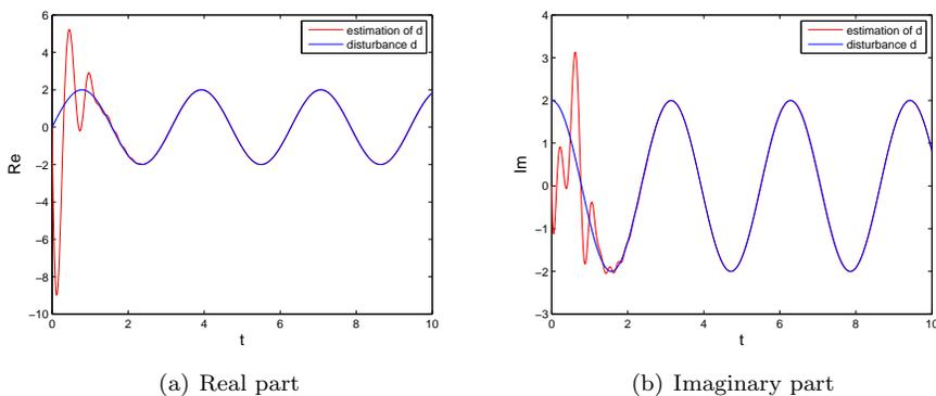
FIGURE 3. The  $\hat{d}(t)$  and disturbance  $d(t) = 2\sin(2t) + 2j\cos(2t)$  by time varying gain
