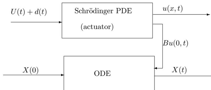
FIGURE 1. Block diagram for the coupled ODE-PDE system
