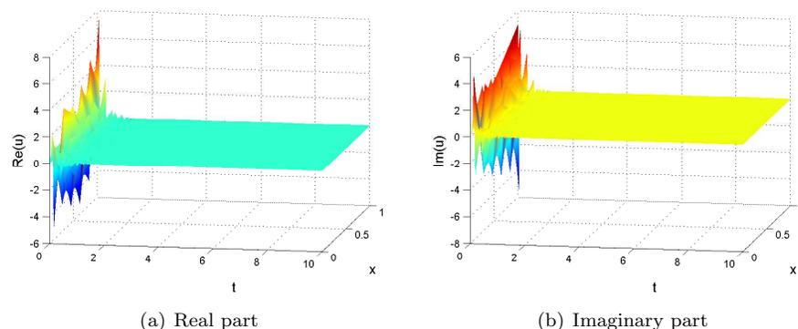
FIGURE 5. The Schrödinger state  $u(x, t)$  with constant high gain controllers
