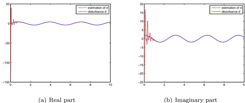
FIGURE 2. The  $\hat{d}(t)$  and disturbance  $d(t) = 2\sin(2t) + 2j\cos(2t)$  by constant high gain
