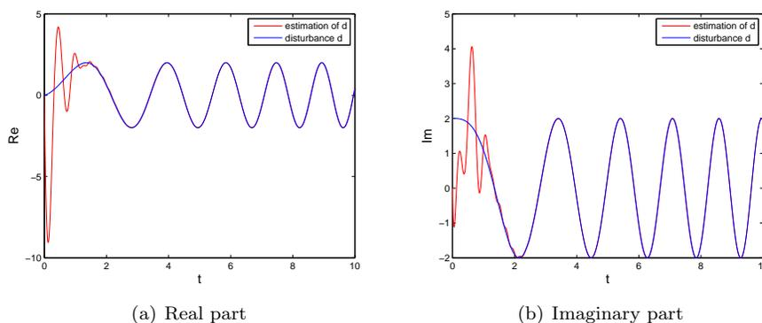
FIGURE 7. The  $\hat{d}(t)$  and the disturbance  $d(t) = 2 \sin(t^{3/2}) + 2j \cos(t^{3/2})$  by time varying gain
