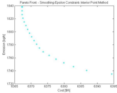
Figure 4: Pareto Front using Smoothing- $\epsilon$ -constraint - Interior point method for  $\mu = 0.01$
