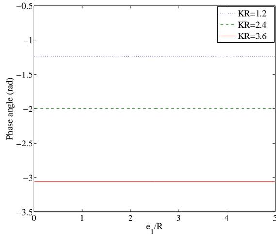
Figure 7: Phase angle of the force  $F_c/\mu$ , against  $e_1/R$  for different values of wave number with fixed  $R = 1.2$  metre.
