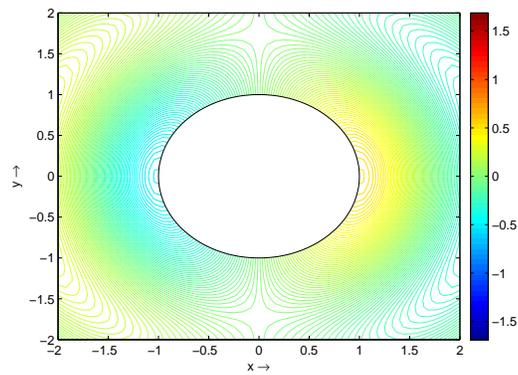
Figure 10: Contour plot for wave elevation in exterior region with  $R = 1.0 \text{ metre}$ ,  $K = 2.5493 \text{ metre}^{-1}$ ,  $t = 1.2566 \text{ s}$ ,  $\theta = 0$ ,  $m = 1$ .
