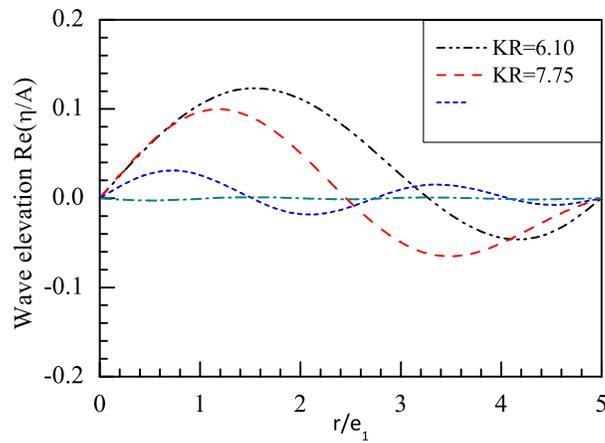
Figure 8: Free surface elevation in the interior region for different wave numbers with  $R/e_1 = 6.25$ ,  $e_1 = 0.8$  metre,  $\theta = 0$ ,  $m = 1$ .
