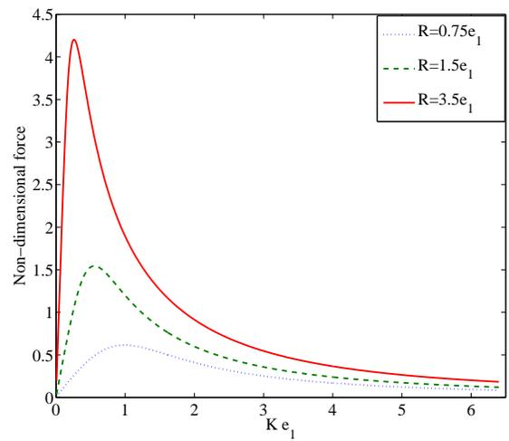
Figure 4: Non-dimensional force  $F_c/\lambda$ , versus wave number for different values of the radius of the cylinder with fixed draft  $e_1 = 0.8$  metre.
