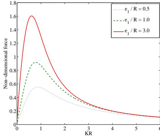
Figure 2: Non-dimensional horizontal exciting forces ( $F_c/\mu$ ) versus  $KR$  for different values of draft of the cylinder with fixed radius  $R = 1.2$  metre.
