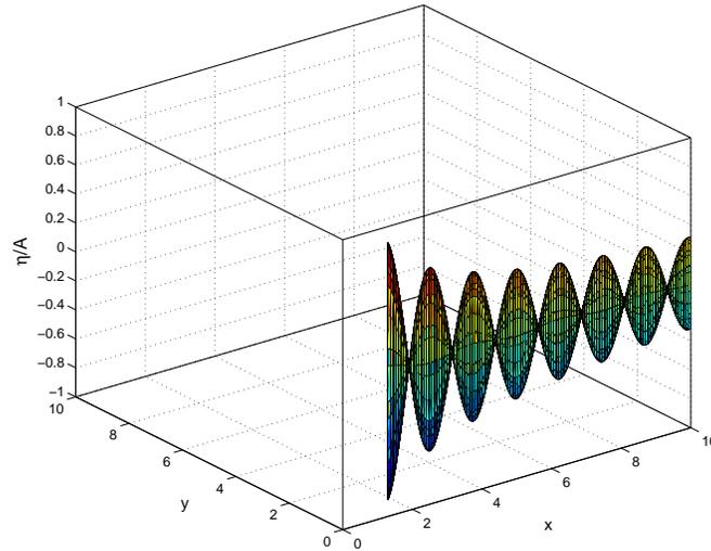
Figure 9: Surface plot for wave elevation in exterior region with  $K = 2.5493 \text{ metre}^{-1}$ ,  $\theta = 0$ ,  $m = 1$ .
