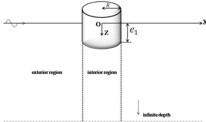
Figure 1: Schematic diagram and definition of fluid subdomains
