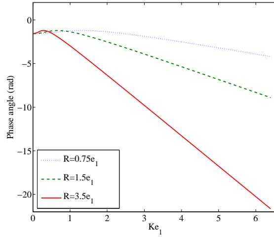
Figure 5: Phase angle of the force  $F_c/\lambda$ , versus wave number for different values of the radius of the cylinder with fixed draft  $e_1 = 0.8$  metre.
