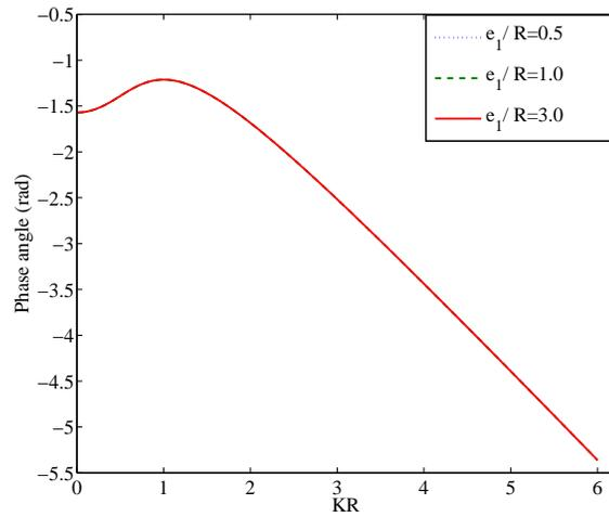
Figure 3: Phase angle of the force  $F_c/\mu$ , versus wave number for different values of draft of the cylinder with fixed radius of the cylinder  $R = 1.2$  metre.
