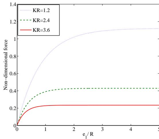
Figure 6: Non-dimensional exciting forces versus draft of the cylinder for different values of wave numbers with fixed radius of the cylinder  $R = 1.2$  metre.
