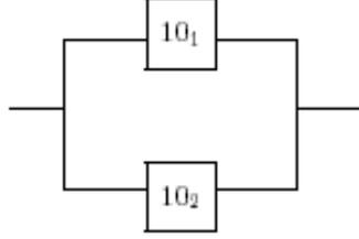
Figure 1: One 10 MW Components with One Standby components
