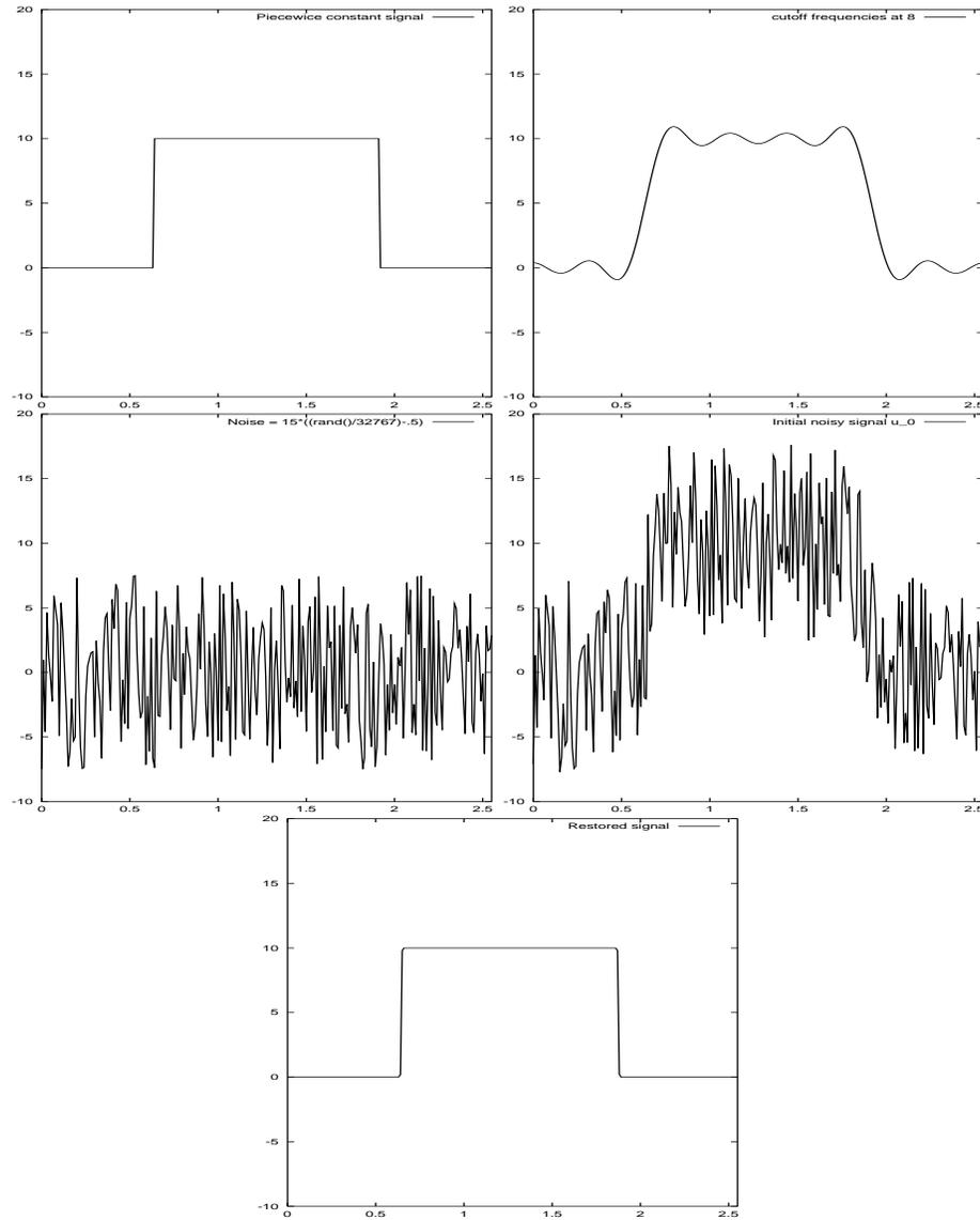
Figure 1: (Top-Left) Initial piecewise signal. (Top-Right) Cutoff frequencies at  $\xi \leq 8$ . (Middle-Left) noise. (Middle-Right)  $u_0 = (\text{Top-Right}) + \text{noise}$ . (Down) Signal  $u_0$  restored and quantized by our model.
