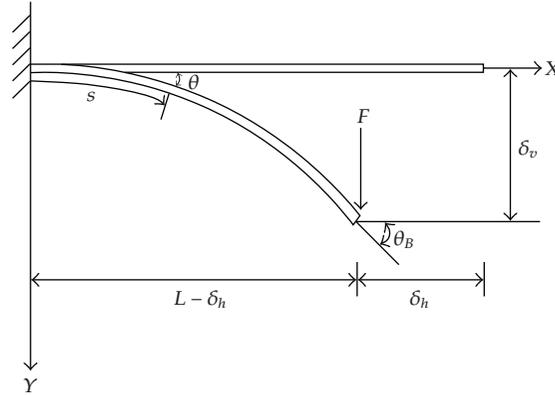
Figure 1: Cantilever beam subjected to a free end point loading.
