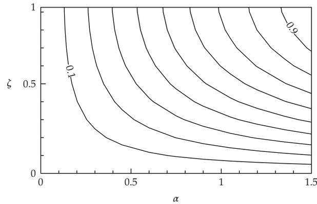
**Figure 3:** The dimensionless normalized rotation angle of the beam versus  $\alpha$  and  $\zeta$  with respect to a reference value of 0.644930, for  $\alpha$  from 0 to 1.5, and  $\zeta$  from 0 to 1.
