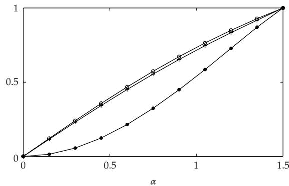
**Figure 4:** The dimensionless normalized (+) rotation angle (o) vertical and (•) horizontal displacements of the beam at free end point versus  $\alpha$  from 0 to 1.5; the references values are 0.644930, 0.410876 and 0.104729, respectively.
