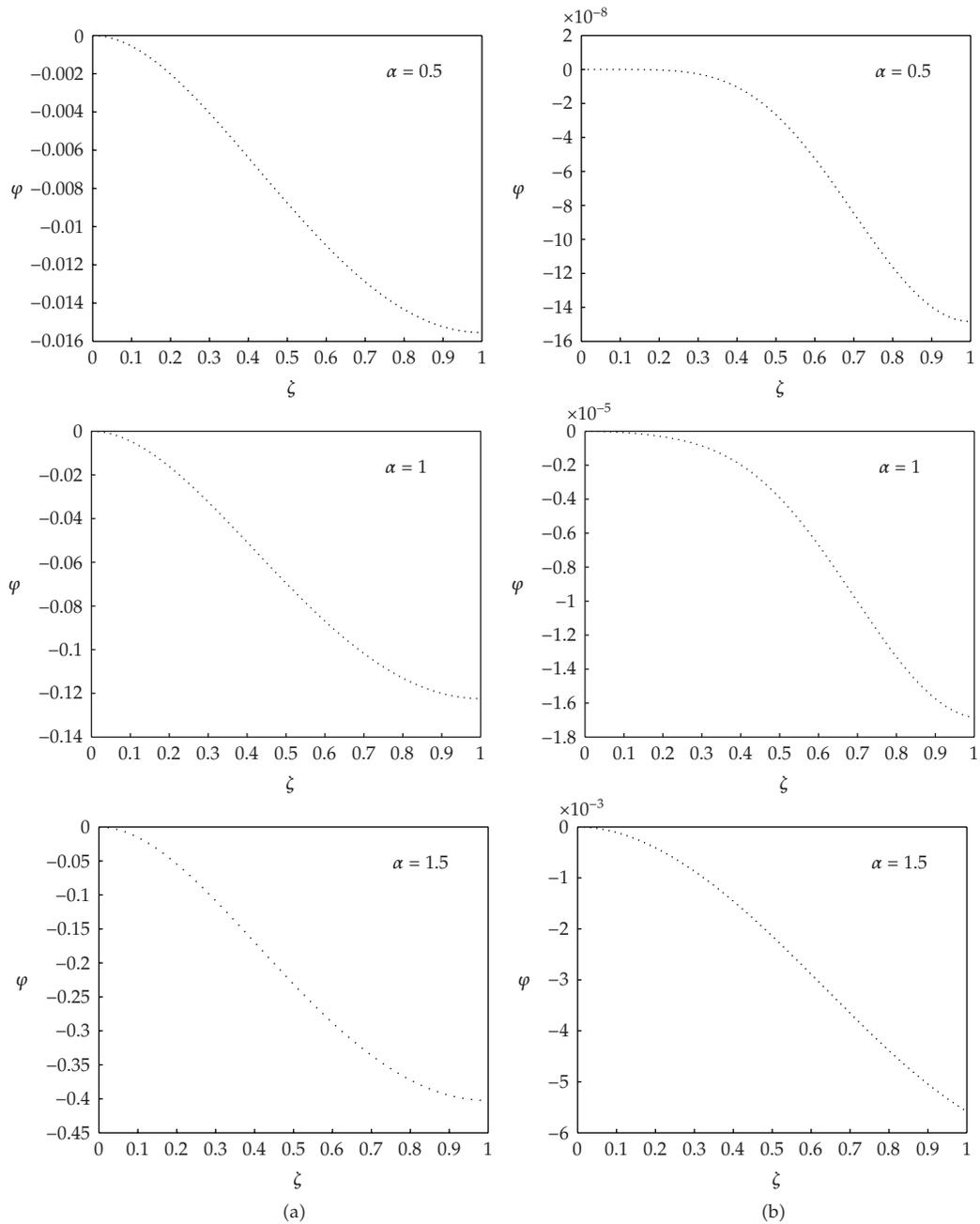
Figure 2: The residual of rotation angle versus  $\zeta$  from (a) linear solution and (b) presented method.
