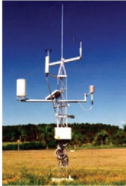
**Figure 1:** Typical meteorological data collection platform.
