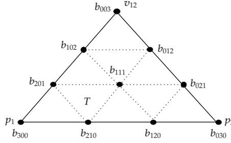
Figure 1: The control points of a Bézier triangle patch of degree three.
