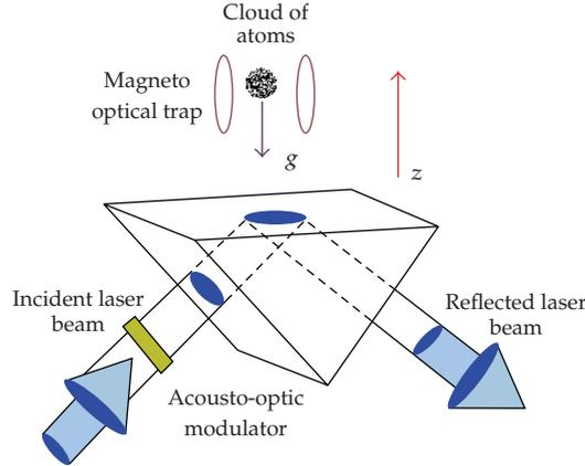
**Figure 1:** A cloud of atoms is trapped and cooled in a magneto-optical trap up to a few micro-Kelvin. The magneto-optical trap (MOT) is placed at a height at the start of the experiment. On switching off the MOT, atoms move with constant gravitational acceleration towards the exponential decaying field.
