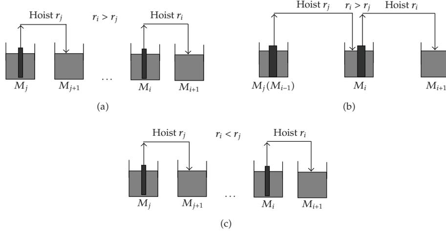
**Figure 5:** (a) No collisions in the execution of two moves ( $r_i > r_j$ ,  $i > j + 1$ ). (b) Execution of two moves requires using a boundary tank  $M_i$  ( $r_i > r_j$ ,  $i = j + 1$ ). (c) Execution of two moves requires using an overlapping zone of the track from  $M_j$  to  $M_{i+1}$  ( $r_i < r_j$ ,  $i > j$ ).
