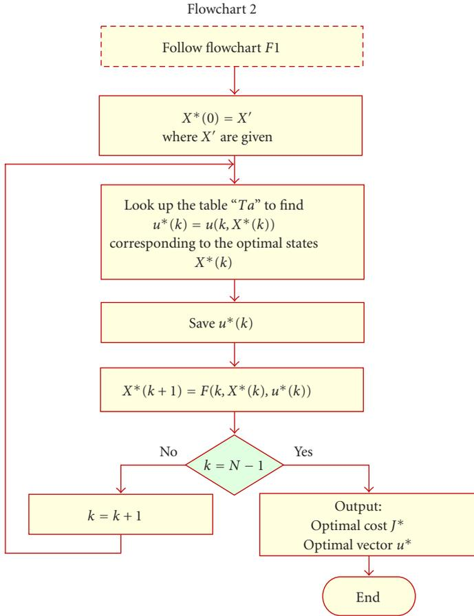
Figure 3.3. Optimal control token-bucket algorithm flowchart (part 2).
