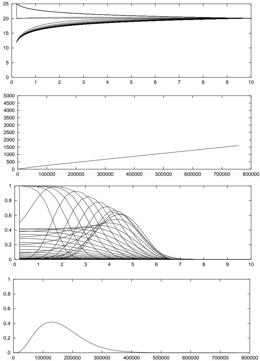
**Figure 4.** Simulation results of the direct problem in injection/extraction: (from top to bottom) successive profiles of hydraulic head (m) vs. radial coordinate (m); total amount of water extracted vs. time (s) during the extraction regime; successive profiles of contaminant concentration vs. radial coordinate (m); contaminant concentration at  $r = r_0$  vs. time (s) during the extraction regime.
