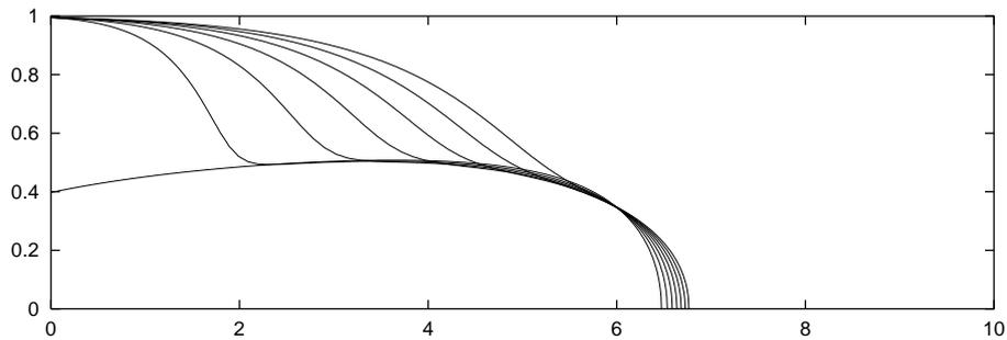
**Figure 3.** Subsequently saturation distribution under gravitation, after 0, 600, 1200, ..., 3600 seconds.
