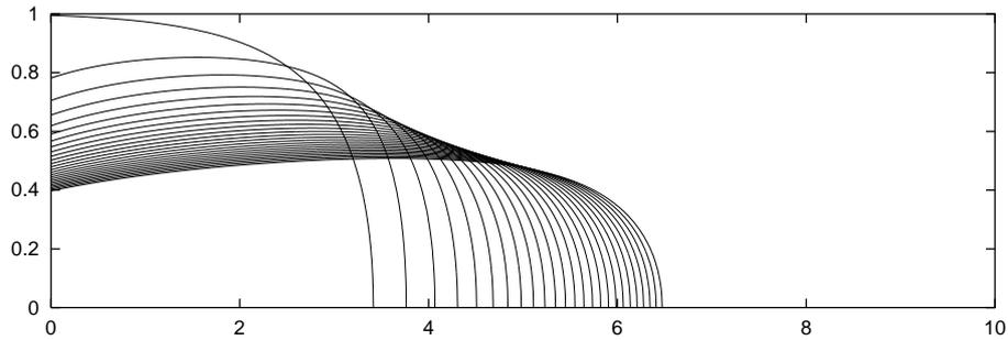
**Figure 2.** Subsequent saturation distribution in the sealed centrifugation, after 0, 600, 1200, ..., 14400 seconds.
