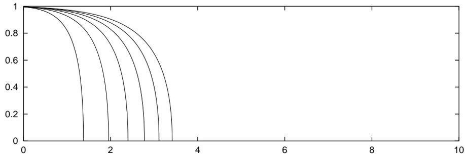
**Figure 1.** Saturation distribution along sand sample (of 10 cm length) under gravitation, after 600, 1200, ..., 3600 seconds.
